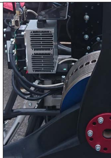
The Geiger double motor is redundant throughout.
