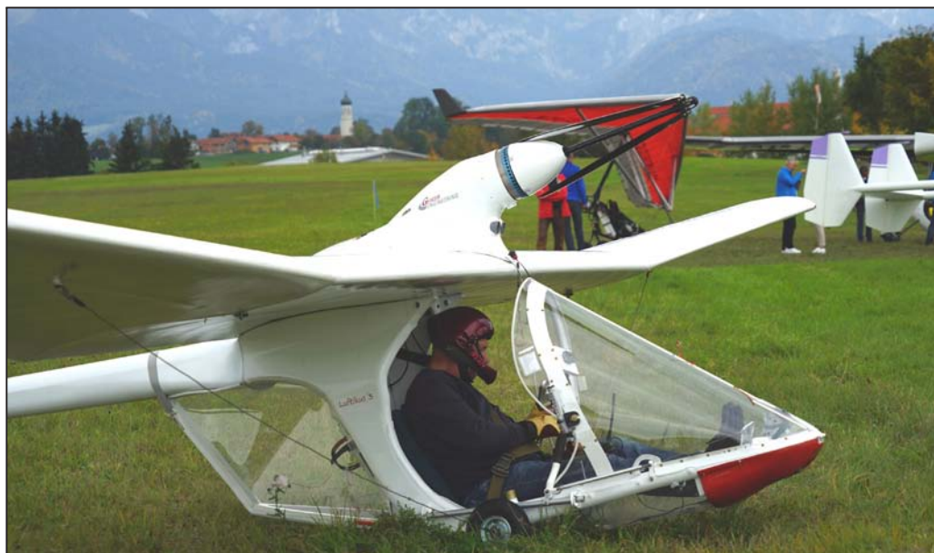
This homebuilt airplane with single-disc electric motor from Geiger has good gliding characteristics.
