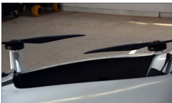
Large overlapping propellers for low Noise levels.
