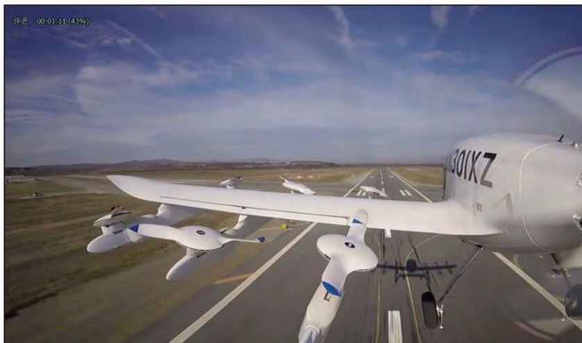
A close look at the rotor and boom indicates that the rotors are tilted toward different directions.
