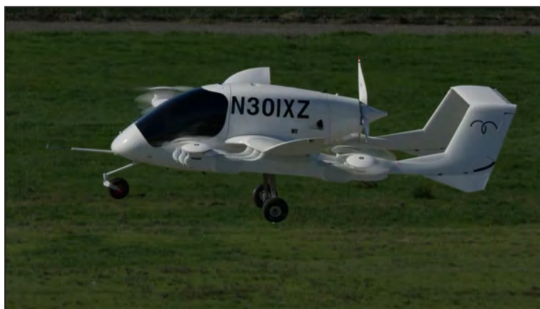
Cora has conventional fixed wing airplane layout with twin boom fuselage, pusher propeller and tricycle landing gear. The rotors on the booms providing VTOL lift make all the difference.
