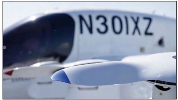
The rotor blade has short length and long chord.
