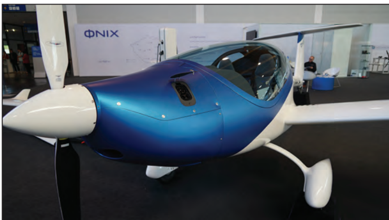
U15 e uses MGM COMPRO RE80 electric motor.
