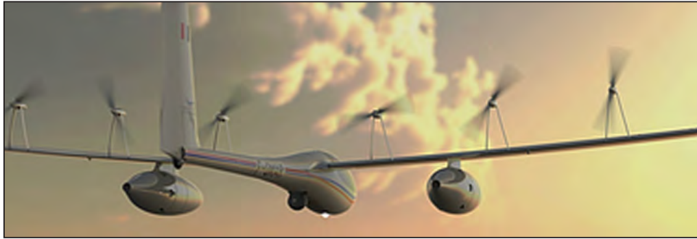
Lange Research E2: 40 hours flight with fuel cells
